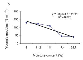
Fig. 6. Effect of temperature (a) and moisture content (b) on Young's modulus.
