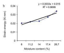
Fig. 5. Effect of temperature (a) and moisture content (b) on strain energy.
